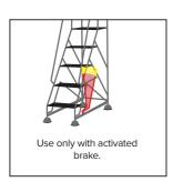
If not a spring-loaded step, then the brake bar must be in the retracted position prior to ascending the steps – i.e: the step must not be in the mobile mode where all 4 castors/wheels are in contact with the ground.
