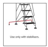
For steps that are fitted with stabilisers – the stabilisers must be in the fully extended position prior to ascending the steps.
