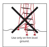
Use only on firm level ground. Surface should be sound and smooth – rough /uneven surfaces could cause the steps to be unstable. Moving the steps around on rough/uneven ground could also cause damage to the castors and footpads.
