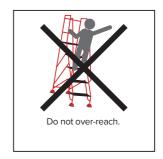
In proper use the platform is stable. Operatives should be instructed not to lean over the rail. Operatives should stand central to the top platform and work within arms distance of products or maintenance etc.
